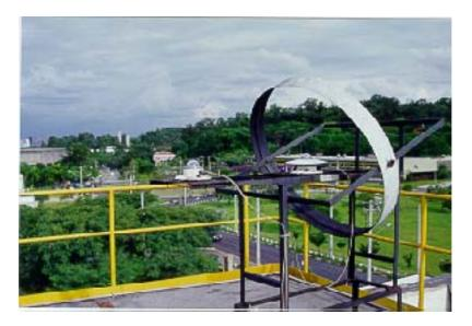
**Figure 2a:** The *IAG site* in the University of São Paulo Campus, São Paulo (23<sup>°</sup>32'S). The shadow-band device has 40 cm of diameter. The picture reports the Southeast sector of the University Campus, with the Oceanographic Institute behind.
