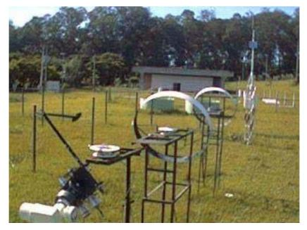
**Figure 2b:** The *UNESP site* in the State University of São Paulo, Botucatu, SP (22<sup>°</sup>51'S). Both shadow-band devices have 40 cm of diameter. The solar tracker in the up front has a shadow disk coupled in it. The picture reports the Southeast sector the State University of São Paulo campus located at left side of the Department of Environmental Sciences building.
