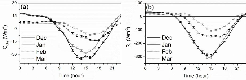
Figure 1. Average diurnal variation of (a) soil heat flux ( $G_{obs}$ ) and (b) net all-wave radiation ( $R_n$ ) for summer period (DJFM) of 2013/2014. The vertical bars indicate the statistical error.
