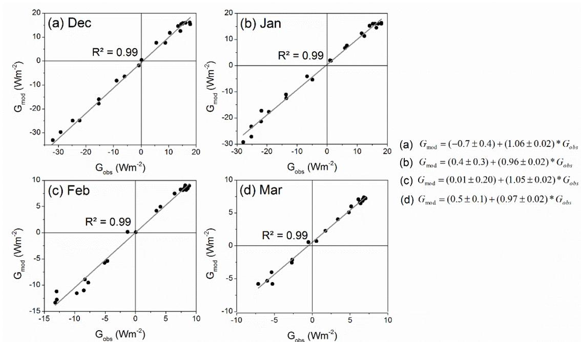
Figure 3. Soil heat flux ( $G_{\text{obs}}$ ) observed vs modelled ( $G_{\text{mod}}$ ) using the OHM method for summer period 2013/2014 in EACF. (a) December, (b) January, (c) February, and (d) March. The gray straight lines represent the equations on the right side.
