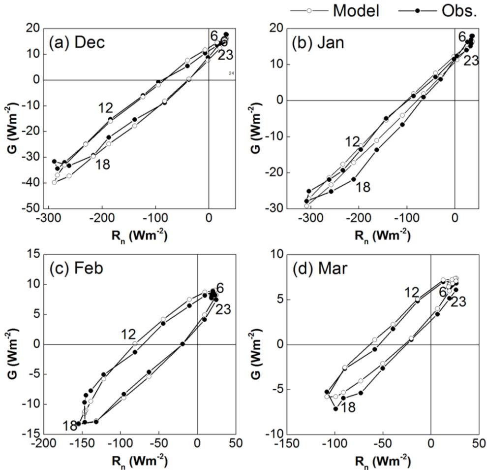
Figure 2. Hysteresis loop relations between soil heat flux ( $G$  - observed and modelled) and net all-wave radiation ( $R_n$ ) for summer period 2013/2014 in EACF: (a) December, (b) January, (c) February, and (d) March. The numbers represent the time (hour).
