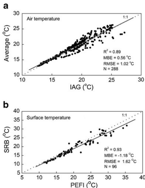
**Fig. 5** Dispersion diagrams comparing hourly values of **a** air temperature measured at the IAG and the average over all the other sites in the city of São Paulo and **b** surface temperature measured at the PEFI and provided by the SRB project during 2004. The linear fit and the diagonal are indicated by *continuous* and *dotted* lines, respectively
