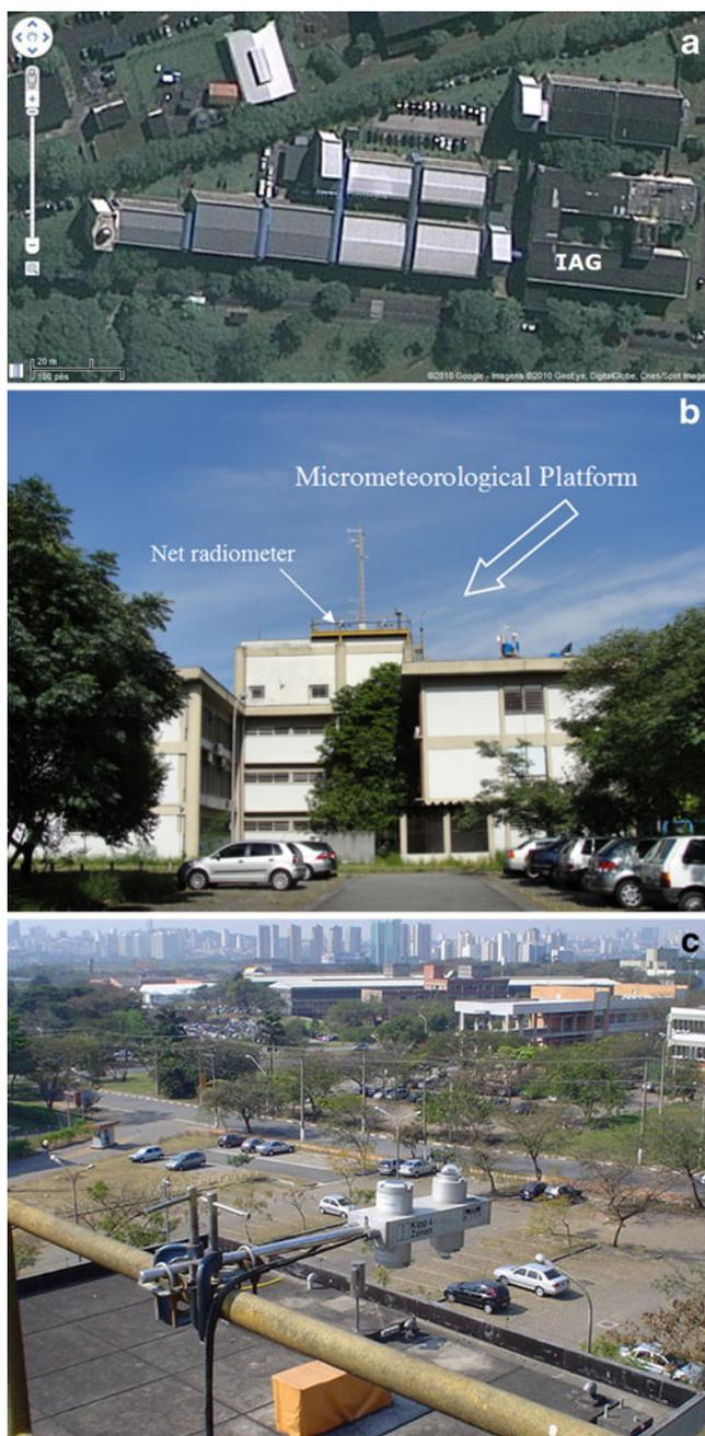
**Fig. 2** a The IAG building, b the micrometeorological platform, and c the net radiometer. The land use of the University of São Paulo campus is classified as suburban. In b, the view is from the parking lot located east of the IAG building
