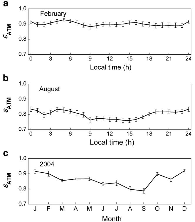
**Fig. 11** Diurnal evolution and seasonal variation of the atmospheric effective emissivity at the surface in **a** February, **b** August, and **c** 2004 at São Paulo. The vertical lines indicate statistical errors
