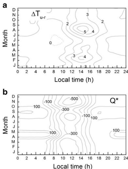
**Fig. 13** Seasonal variation of the diurnal evolution of **a** UHI intensity (degree Celsius) and **b** net radiation (watts per square meter) at the surface in the city of São Paulo during 2004
