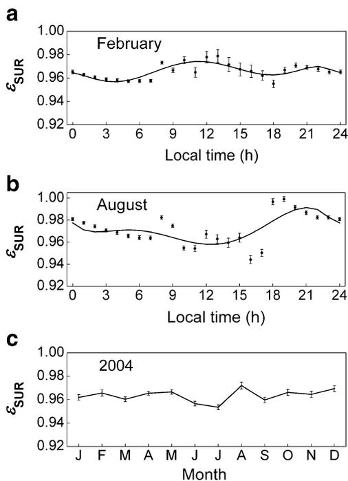
**Fig. 12** Diurnal evolution of the surface emissivity during **a** February and **b** August and **c** seasonal variation at São Paulo. Continuous lines in **a** and **b** indicate the sixth-order polynomial fit. The vertical lines indicate statistical errors
