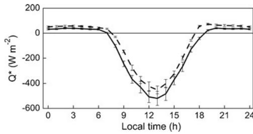
**Fig. 6** Diurnal evolution of net radiation at the surface in the city of São Paulo during February (*solid line*) and August (*dash line*) in 2004. Statistical errors are indicated by *vertical bars*
