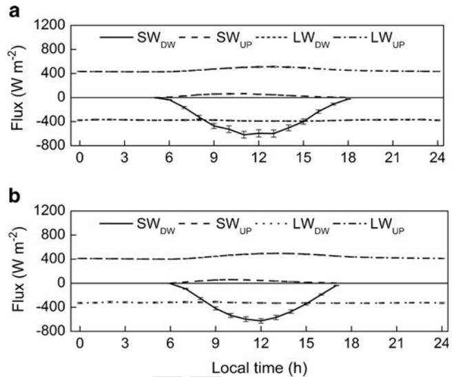
**Fig. 7** Diurnal evolution of the components of the radiation balance at the surface in the city of São Paulo during **a** February and **b** August of 2004. Statistical errors are indicated by *vertical bars*
