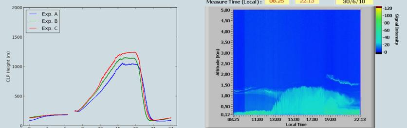
Figure 2: Diurnal evolution of PBL height simulated by LES model (see Table 1) (top left) compared with observed aerosol layer depth by LIDAR on June 30<sup>th</sup>, 2010 (Landulfo *et al.*, 2010) (top right). Both LES simulation and LIDAR observation show a maximum PBL height of 1100-1400 m. The maximum PBL height of 1200 m observed in the radiosonde profiles in a typical clear sky day in São Paulo (June 16<sup>th</sup>, 2010 at 00 GMT), is indicated in the bottom left.
