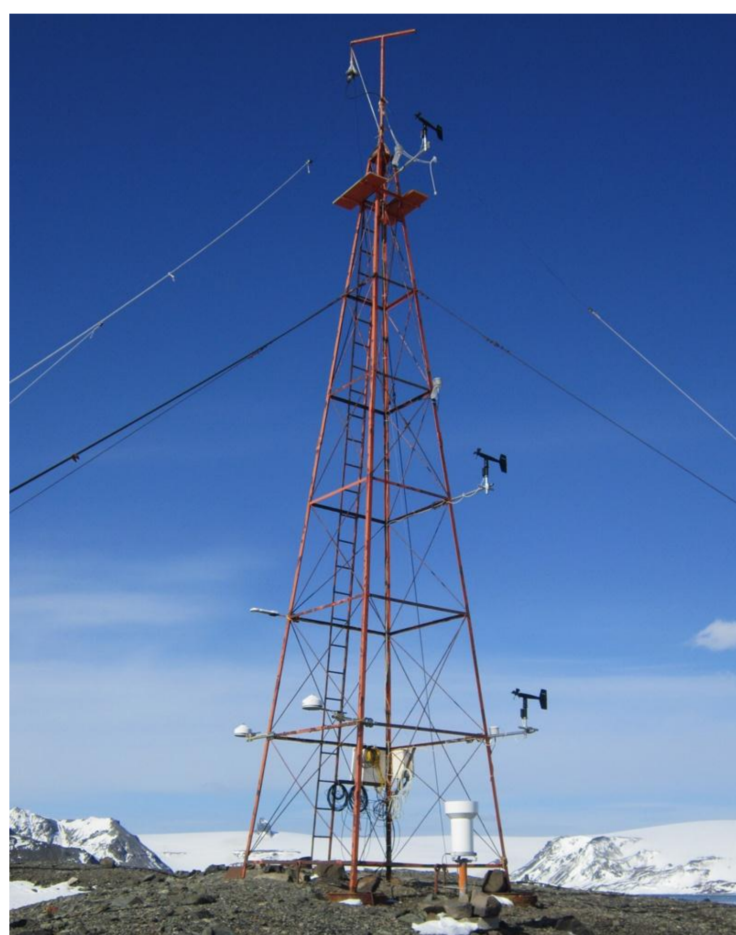
Fig. 5: East view of the 12 meter South Tower instrumented with radiation, wind, air humidity and air temperature sensors.
