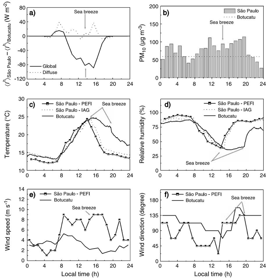
**Fig. 10.** Diurnal evolution of hourly values of (a) difference between solar irradiances in São Paulo and Botucatu; (b) particulate matter in São Paulo and the August average value of Botucatu (dotted line); (c) air temperature in São Paulo (PEFI and IAG) and Botucatu; (d) relative humidity in São Paulo (PEFI and IAG) and Botucatu; (e) wind speed in São Paulo (PEFI) and Botucatu and (f) wind direction in São Paulo (PEFI) and Botucatu. August 24, 1999
