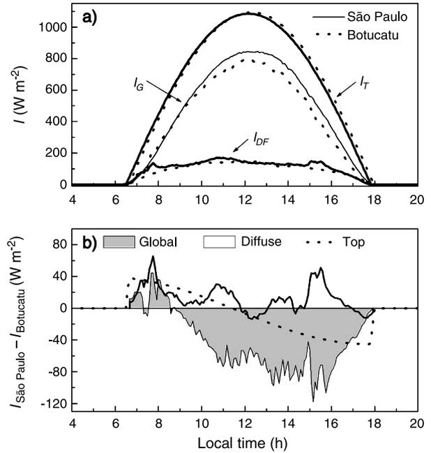
**Fig. 4.** Diurnal evolution of (a) global ( $I_G$ ), diffuse ( $I_{DF}$ ) and extraterrestrial solar irradiance ( $I_T$ ) for São Paulo (continuous line) and Botucatu (dotted line) and (b) difference between solar irradiances in São Paulo and Botucatu, August 24, 1999
