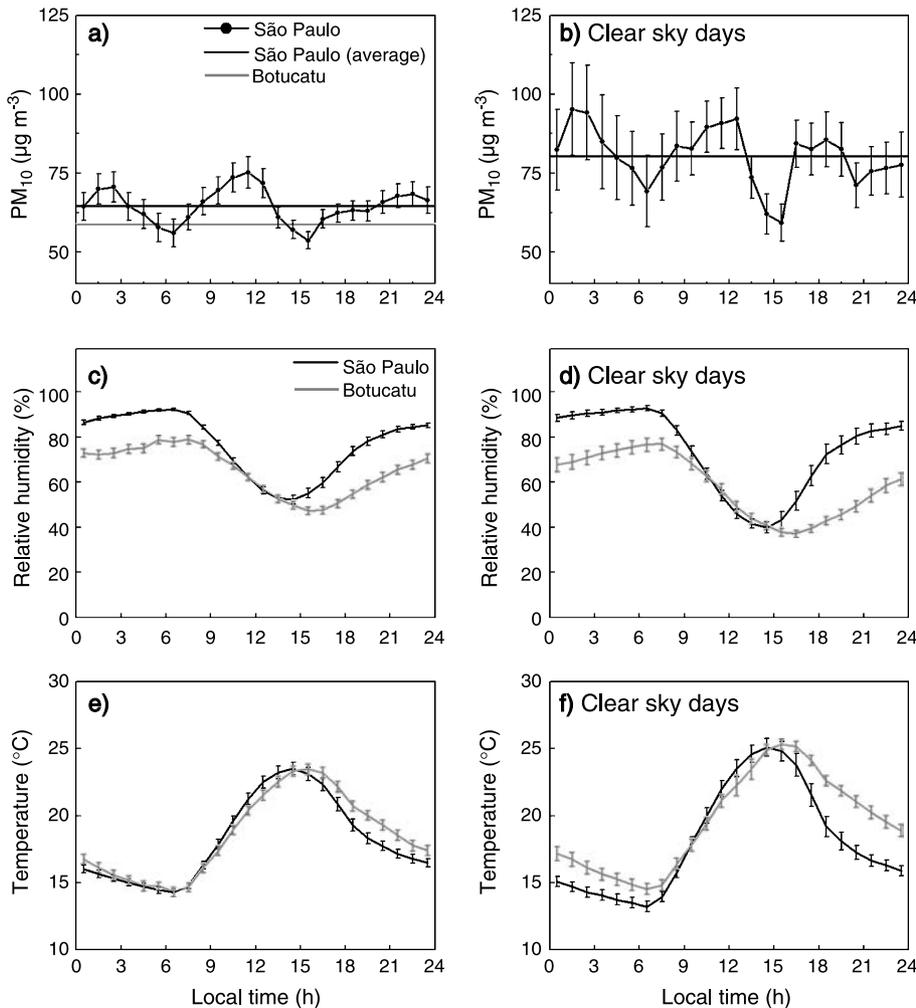
**Fig. 9.** Diurnal evolution of monthly-averaged hourly values of (a, b) particulate matter ( $PM_{10}$ ) measured in São Paulo; (c, d) relative humidity; (e, f) temperature. In (a) and (b) the black thick continuous lines correspond to the 24 h averaged  $PM_{10}$  for São Paulo. The observational period are indicated in Table 1. Vertical bars correspond to the error values
