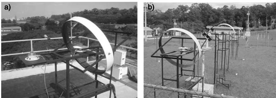
**Fig. 2.** The shadow-band devices, with 40 cm of diameter, used to measure diffuse solar irradiance at (a) IAG site in São Paulo and (b) Botucatu
