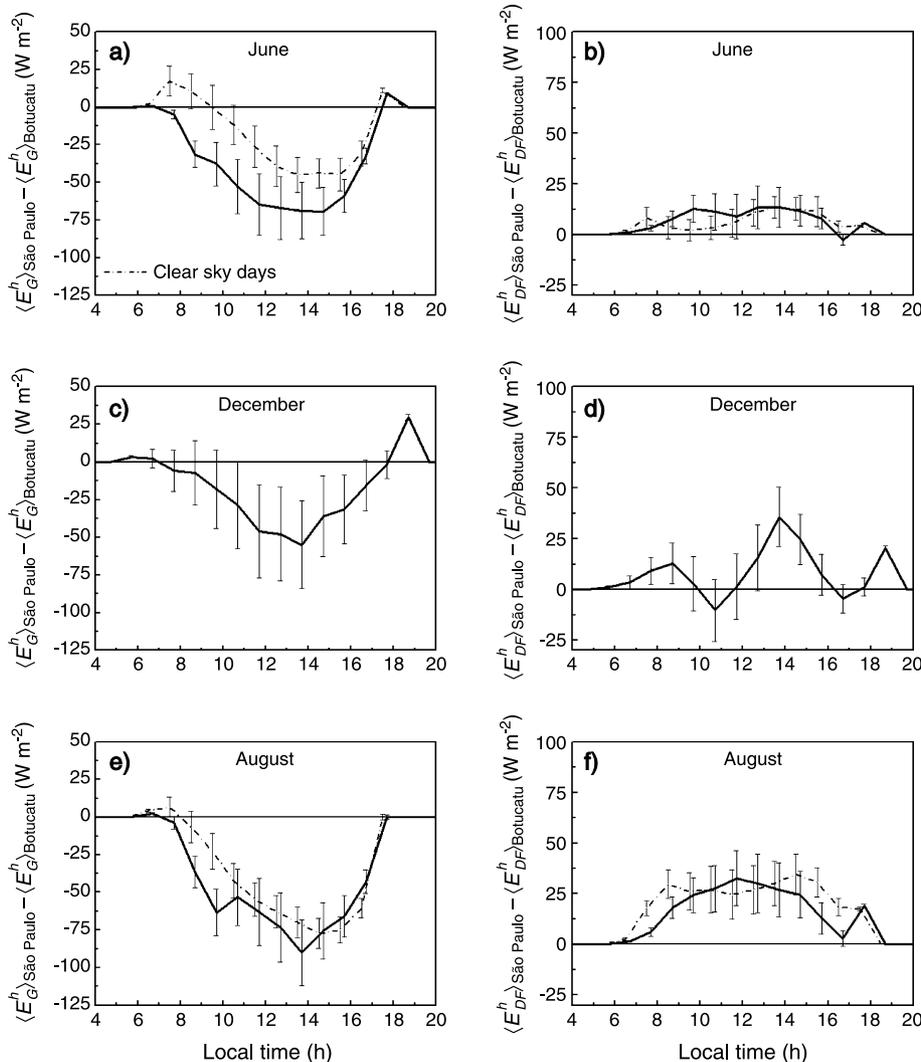
**Fig. 8.** Diurnal evolution of monthly-averaged hourly values of global and diffuse solar irradiance differences between São Paulo and Botucatu (continuous line) and clear sky days (dashed line). June, December and August (1996–2001). Vertical bars correspond to the error values
